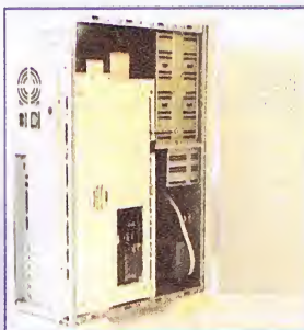
The EZPC Tower system showing the A1200, the PC rear sockets, card slots and removable side panels
